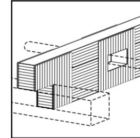
Design of notches or openings based on structural analysis. Machining by the glulam manufacturer or after consultation with the engineer.
