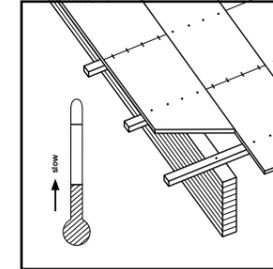
Fast covering of the building avoids high moisture content of the wooden product and resulting cracks during drying. Heating the building must be done slowly.
