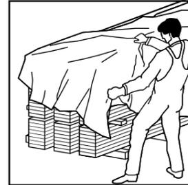
Protect the timber against absorbing humidity by covering it. Remove or check the transport packaging immediately to avoid condensation risk.
