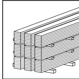
Use dunnage bars for stacking to protect the timber against tilting. To prevent deformations, the dunnage bars should always be arranged in line above the other.
