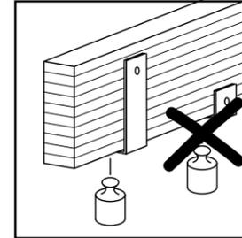
Additional loads have to be approved with an appropriate structural analysis. Avoid any tensile stress perpendicular to the grain.
