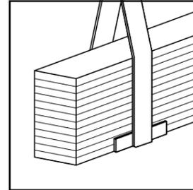
Use broad lifting straps and edge protectors to avoid damages. Prepare the correct lifting tool and protection measures in regards to the material, package size, etc. you have to move.
