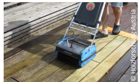
Cleaning of terrace surfaces using a brushing machine.
